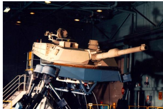
Figure 1: Crew Station Turret Motion Base Simulator outfit with heavy turret system.
